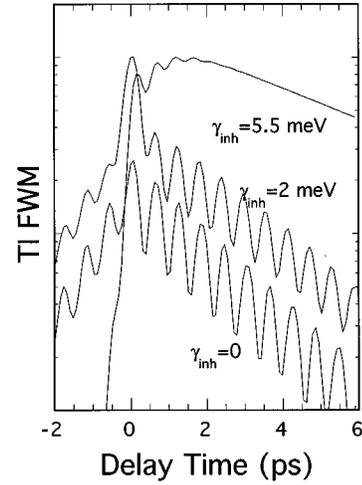
FIG. 7. Time-integrated (TI) FWM signals, emitted at the lower polariton energy, calculated for different inhomogeneous  $X$  linewidths  $\gamma_{\text{inh}}$ , and for zero detuning  $\Delta$ . Other parameters are given in the text.
