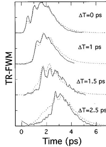
FIG. 4. Experimental (solid) and theoretical (dashed) time-resolved (TR) FWM signals for different delays  $\Delta T$  in the  $\parallel$  polarization geometry. Detuning  $\Delta = -2$  meV, and  $I_{\text{ex}} \approx 3 \times 10^{11}$  photons/(pulse  $\text{cm}^2$ ). At  $t = 0$  the second pulse impinges on the sample.
