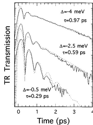
FIG. 2. Time-resolved (TR) transmission, measured (solid curves) at different detunings  $\Delta$  between cavity and exciton. The dashed curves represent the numerical solutions of the Maxwell equations, as explained in the text.  $\tau$  is the exponential decay time.
