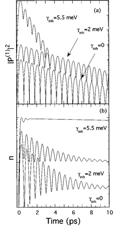
FIG. 5. (a) Square modulus of the linear polarization,  $|P^{(1)}|^2$ , and (b) exciton population  $n$ , vs time after excitation by a 100-fs-wide laser pulse, calculated at resonance ( $\Delta=0$ ) and for different inhomogeneous  $X$  linewidths  $\gamma_{\text{inh}}$ . Other parameters are given in the text.
