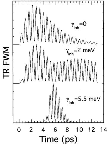
FIG. 6. Time-resolved (TR) FWM signals, calculated for different inhomogeneous  $X$  linewidths  $\gamma_{\text{inh}}$ , for  $\Delta=0$  and  $\Delta T=5$  ps. At  $t=0$  the second pulse impinges on the sample. Other parameters are given in the text.
