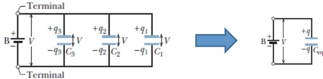
$$q_1 = C_1 V, \quad q_2 = C_2 V, \quad \text{and} \quad q_3 = C_3 V.$$
