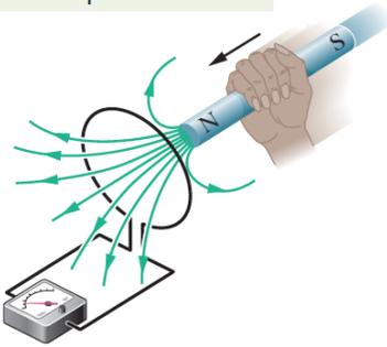
The magnet's motion creates a magnetic dipole that opposes the motion.
