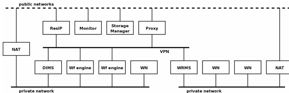
Figure 10. Schema of network connectivity.
