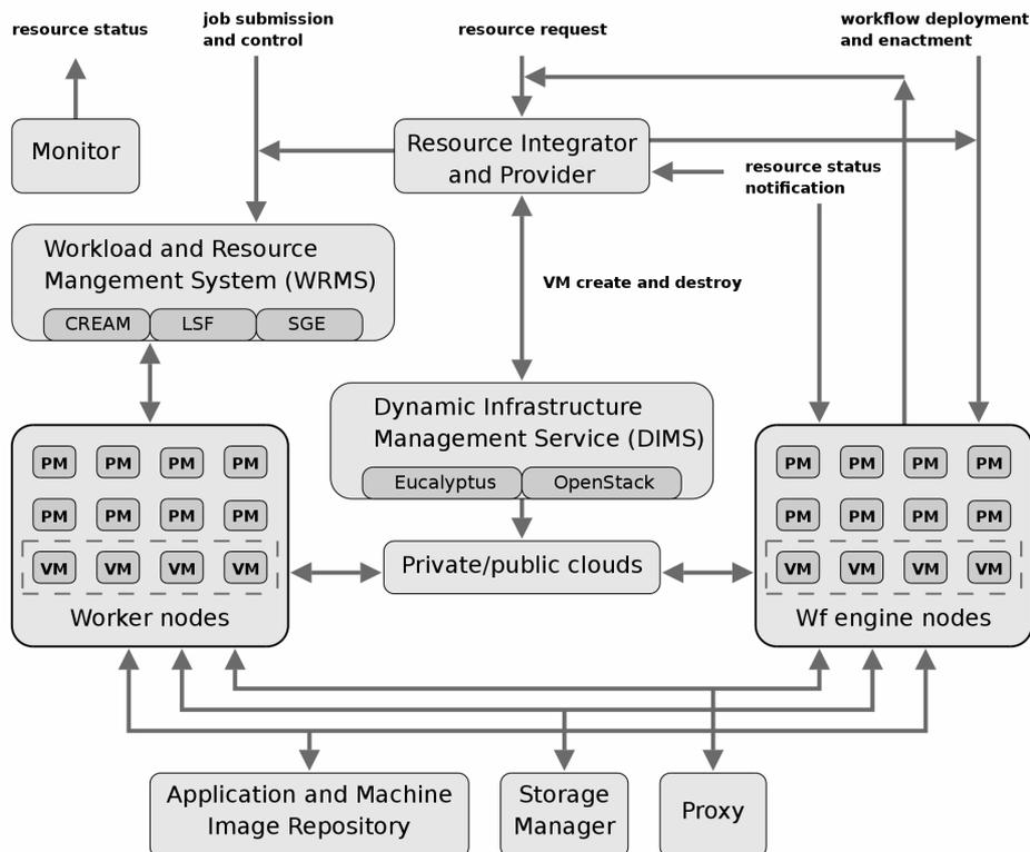
Figure 4. Model of dynamic on-demand resource provisioning system.
