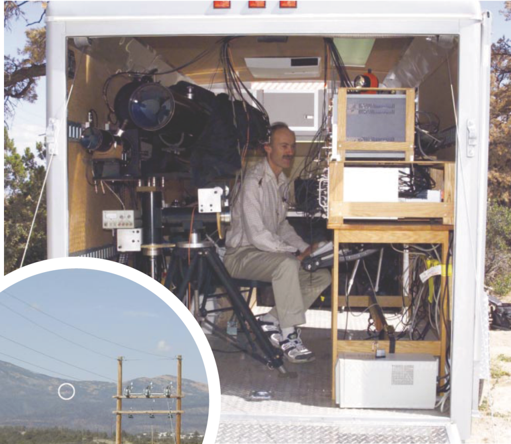
In the air: Richard Hughes has sent a photon-encrypted code from a laser source (circled, inset) to a receiver.
