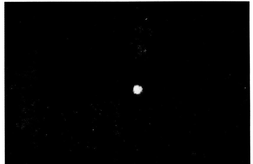
Plate II. – Optical molasses for sodium atoms is seen as a bright area at the intersection of three pairs of centimeter diameter, counterpropagating laser beams. The additional laser beam above the molasses decelerates the atomic sodium beam so the atoms are slow enough to be captured by the molasses (photo courtesy of NIST).
