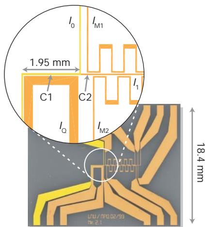
**Figure 1** Atom chip. Bose–Einstein condensates (BECs) were created in magnetic traps formed by tiny gold wires that were created lithographically on a substrate<sup>16,17</sup>. The figure shows the pattern used by researchers at the Ludwig-Maximilians University in Munich<sup>17</sup>. Atoms were trapped at positions C1 and C2.
