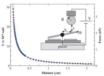
Fig. 2. Angle of rotation  $\theta$  of the top plate and the attractive electrostatic force as a function of distance (23). The red line is a fit obtained with Eq. 7. The voltage V applied to the sphere is 289 mV. (Inset) Schematic of the experiment (not to scale).
