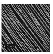
FIG. 1.  $10\times10~\mu m$  AFM topography image of the surface morphology of a p-6P film grown by HWE at 130 °C on mica.
