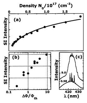
FIG. 3. Panel (a): SI emission intensity vs photoexcited density  $N_0$ , for pump intensities below threshold ( $T=30\,$  K). The solid dots are the experimental points and the solid line is a fit to the data using Eq. (1). Panel (b): SI random lasing plus stimulated emission intensity versus normalized pump excess fluence  $\Delta\Phi/\Phi_{th}$  (T=300 K). Panel (c): Emission spectra recorded at  $\Delta\Phi/\Phi_{th}$ =0.58 and 9.0 (T=300 K).
