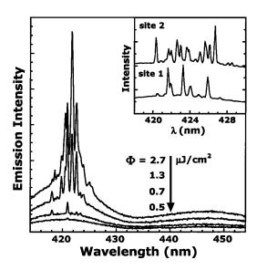
FIG. 2. Main panel: Emission spectra taken at different values of the pump fluence  $\Phi$  ( $\mu$ J/cm<sup>2</sup> per pulse) at T=30 K. Inset: Emission spectra measured in two different positions across the sample surface at the same excitation level above threshold (T = 300 K).
