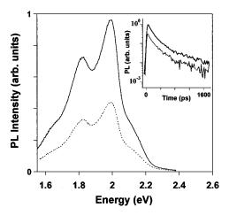
FIG. 6. Polarized PL of a 28 nm-thick film of 4H6T deposited on KAP measured at 84 K (excitation 2.71 eV). In the insert the polarized PL time decay measured at 300 K (excitation 2.33 eV) is reported. The excitation light is polarized along the *b* axis of the KAP. PL is analyzed parallel (solid line) and perpendicular (dashed line) to this direction.
