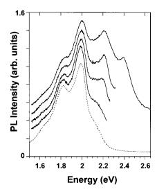
FIG. 4. PL of 4H6T film at  $T=84\,\mathrm{K}$  obtained by exciting at the film edges (solid lines) for different excitations (2.82, 2.45, 2.42, and 2.38 eV from top to bottom). The PL spectrum of the bulk film (dashed line) is reported for comparison (excitation energy 2.75 eV). The PL intensities are normalized and the spectra are displaced vertically for clarity.
