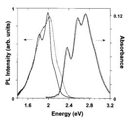
FIG. 3. Absorption and cw photoluminescence spectra of a 28 nm-thick film of 4H6T deposited on KAP at 300 K (dotted line) and 84 K (solid line).
